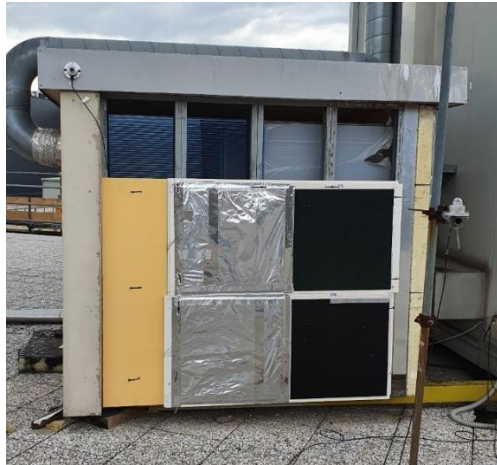
Figure 17. Photograph of the test cell with the screened façade components
