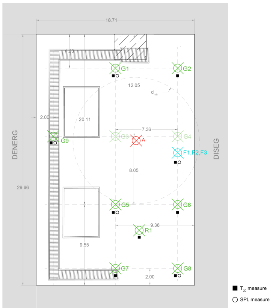
Figure 54. Courtyard plan with the courtyard receiver (in green), the façade receivers (in blue) and source position (in red). The measurement positions in light green are excluded.
