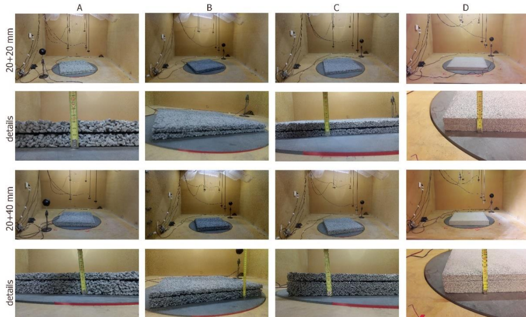
Figure 4. Multiple layers of 20+20 mm and 20+40 mm. Sample A: crushed normal weight aggregates 4-8 mm; Sample B: round lightweight aggregates 4-8 mm; Sample C: round lightweight aggregates 2-4 mm; Sample D: round lightweight aggregates 0.5-1 mm.
