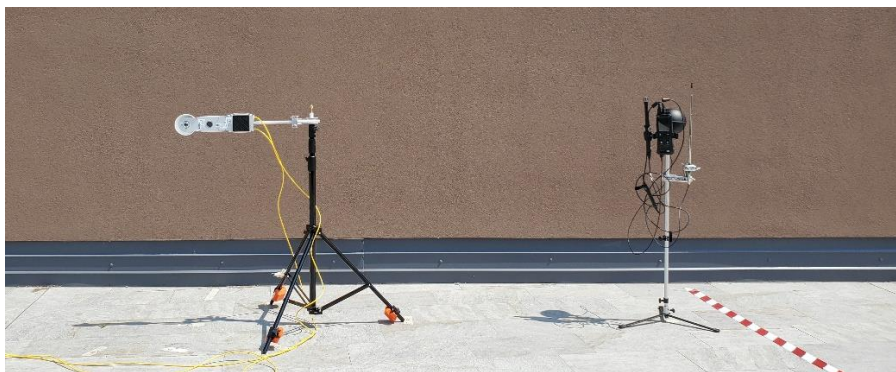
Figure 86. Picture of the measurement equipment, consisting of a single net radiometer (left) and the Testo 480 measuring instrument with the connected sensors (right).
