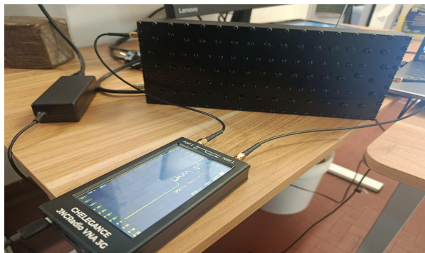
Fig. 8 Diplexer VNA test
