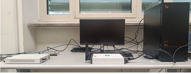
Fig. 1. SDR experimental setup composed of a host computer equipped with MATLAB, a USRP X310 transmitter, and a USRP X410 multi-antenna receiver.
