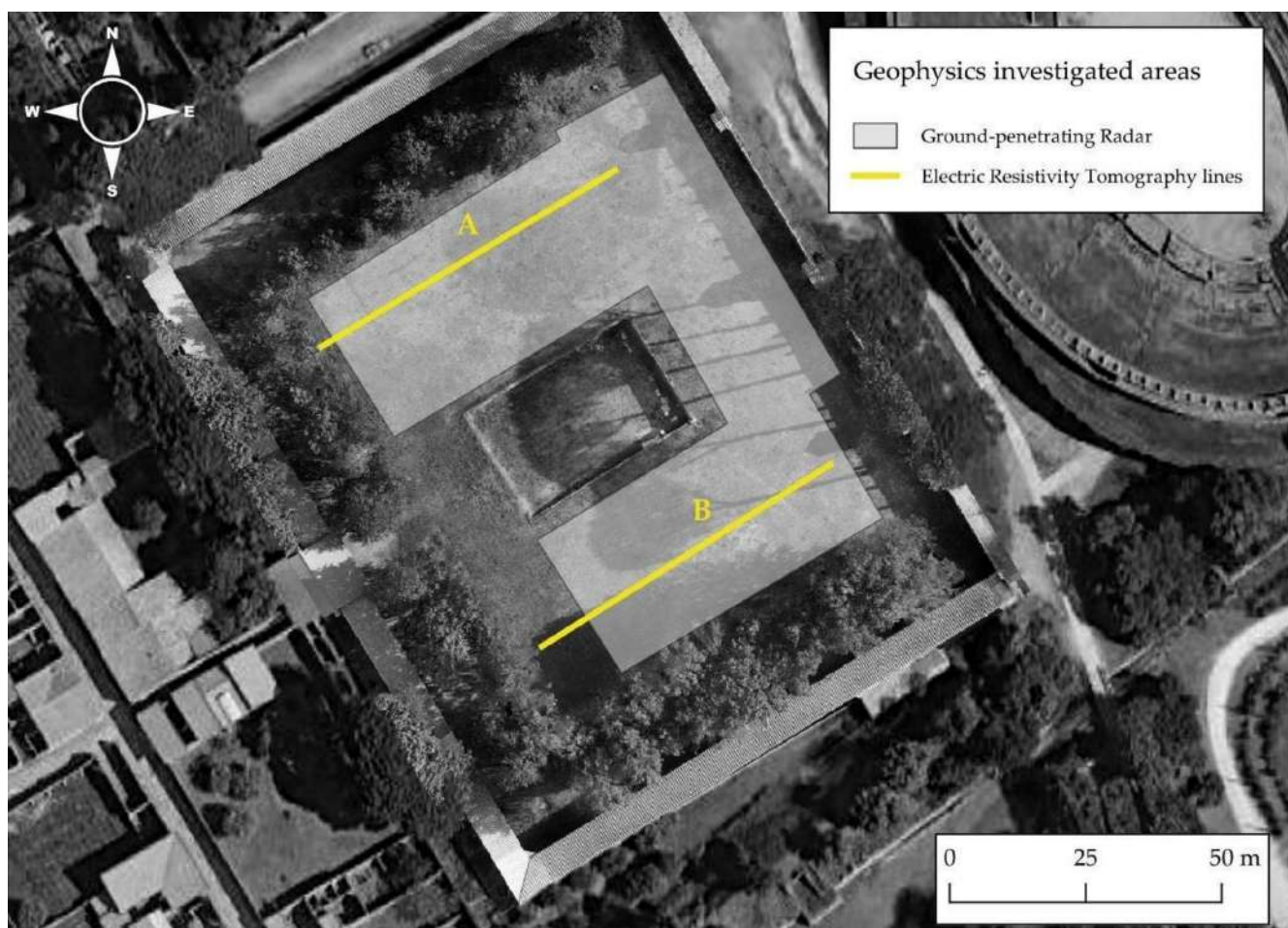
FIGURE 3 | The locations of geophysical surveys conducted in the Palestra Grande . ERT profiles A and B are marked with yellow lines, whereas the grids investigated by GPR are indicated by a white U-shaped polygon.
