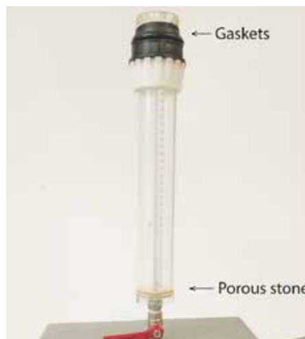
Fig. 6 – Specimen holding cell (left) and detail of the porous stone (right).
