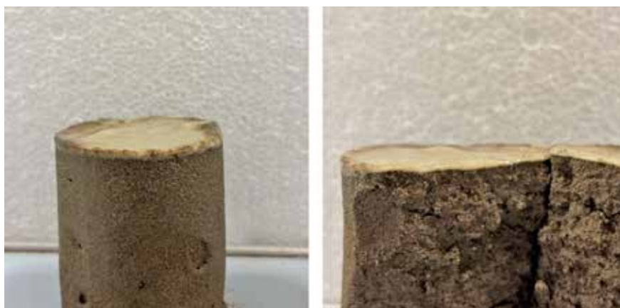
Fig. 7 – Filter cake after filtration test (left), focus on the cake (right).
