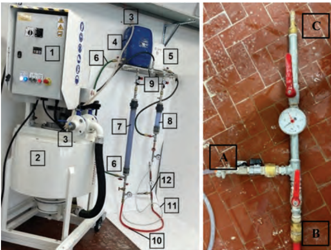
Figure 3. Injection prototype used for the mixing procedure P2. On the left: 1. Mixer control panel for Comp.A production; 2. Mixer + pumping system; 3. Comp.A pumping pipe; 4. Comp.A storage tank; 5. Comp.B storage tank; 6. Comp.A delivery pipe to the pressurization system; 7. Comp.A pressurization pipe; 8. Comp.B pressurization pipe; 9. Compressed air pressurization system; 10. Comp.A delivery pipe to the nozzle; 11. Comp.B delivery pipe to the nozzle; 12. Mixing and injection nozzle. On the right, a detail of the injection nozzle: A. Comp.B feeding line; B. Comp.A feeding line; C: nozzle exit.
