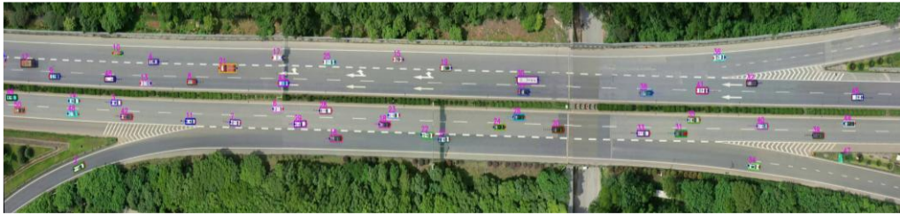
Figure 2.11 The detection performance of the proposed algorithm.
