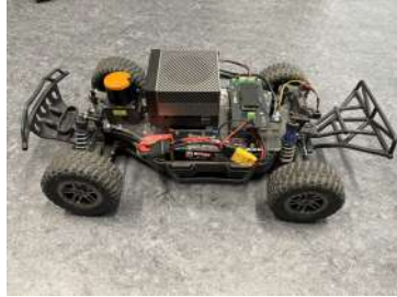
Figure 4: Robotic platform equipped with the Jetson AGX Orin used for deployment.
