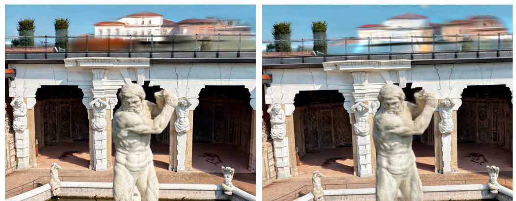
Figure 7. Effect of camera alignment source on PostShot 3DGS reconstruction quality. (Left): external RealityScan camera alignment (1.9M sparse points, 3 min pose estimation). (Right): PostShot internal camera alignment (97.3k sparse points, 13 min pose estimation). Both models use identical 3DGS training parameters: MCMC strategy, 3M maximum Gaussians, 30k iterations.
