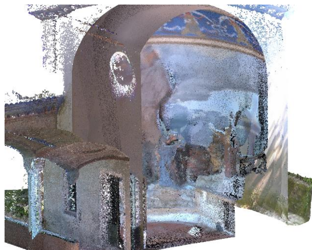
Figure 8. Portion of Stonex X70GO Point Cloud
