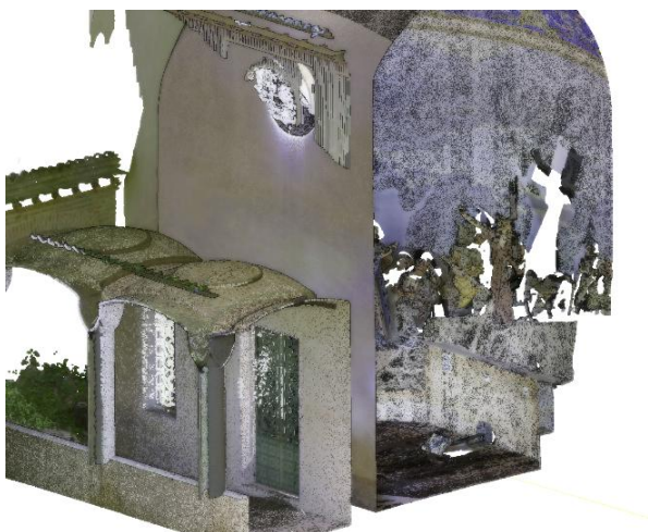
Figure 7. A portion of Leica RTC360 TLS Point Cloud
