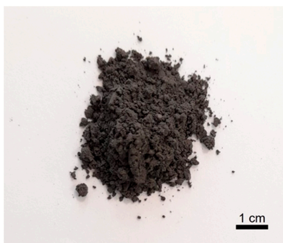
Figure 3. Recycled and sieved NdFeB powder.
