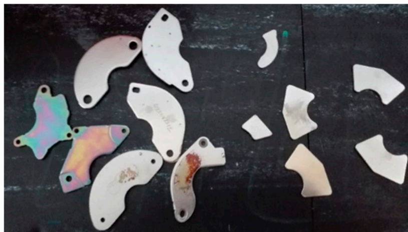
Figure 2. NdFeB magnets ( right ) of different sizes and their magnetic shields ( left ).
