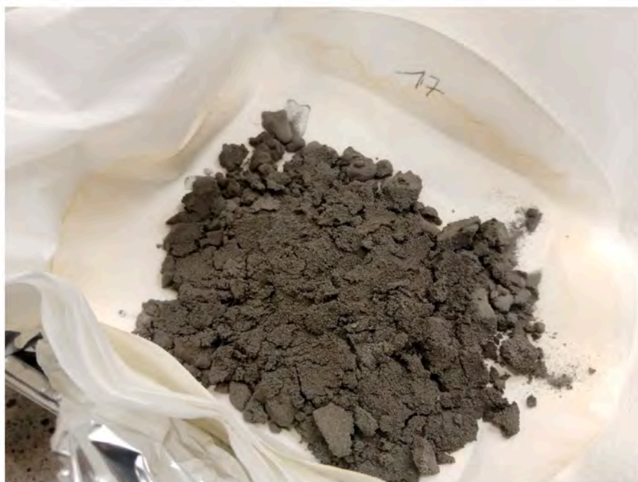
Figure 3. Coated iron powder after the drying phase.
