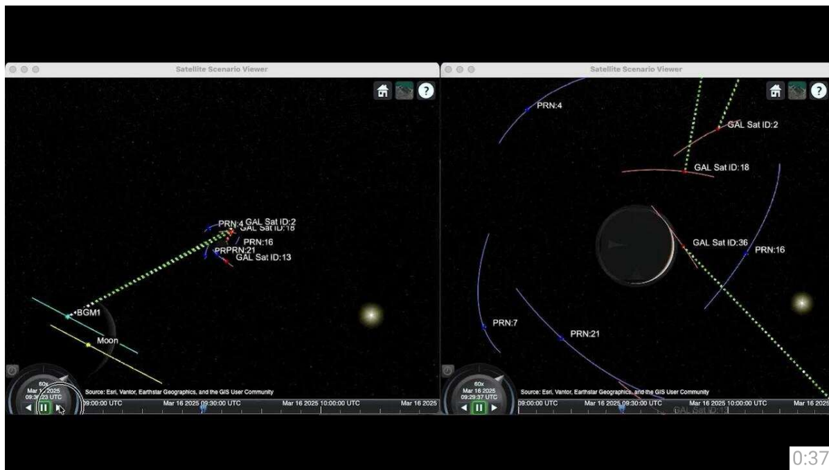
Figure 1. The LuGRE 3D orbital analysis application built using MATLAB, Aerospace Toolbox, Antenna Toolbox™, and Navigation Toolbox™. The application enabled dynamic visualization of the spacecraft, Moon, and GNSS signal paths near the lunar surface (left) and GNSS satellite geometry relative to Earth and the mission trajectory (right).
