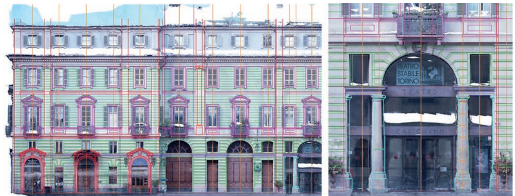
Fig. 5. Survey and graphical analysis superimposed on the orthophoto of the façade of the Carignano Theatre. Elaboration by M. Rinascimento.
