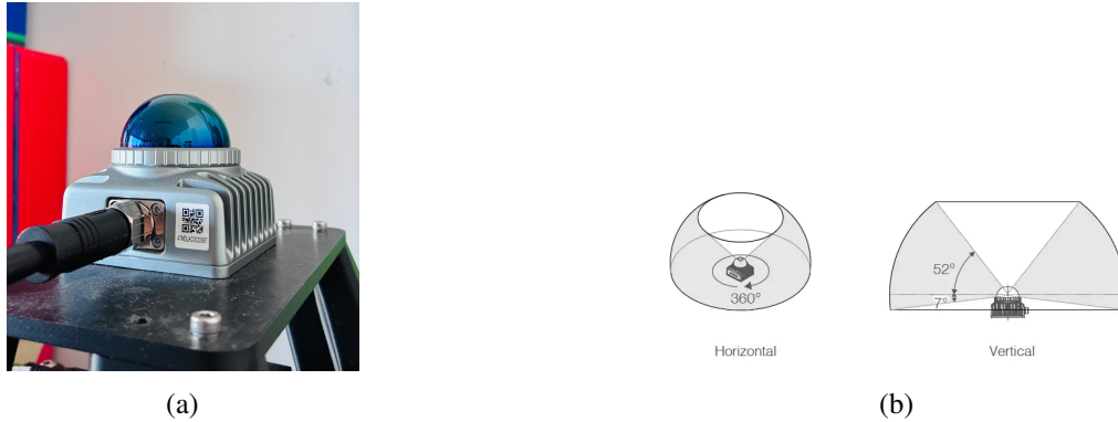
Fig. 4.8 The Livox Mid-360 (a) and its field of view (b)
