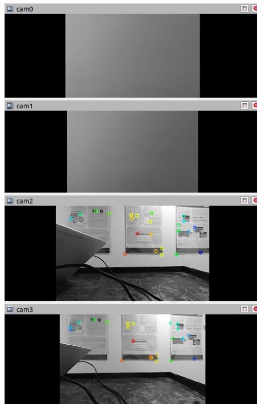
Fig. 3.14 The multi-camera setup during robustness testing: cam0 and cam1 (Stereo 1); cam2 and cam3 (Stereo 2).
