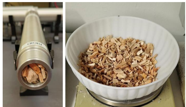
Figure 1. Impedance tube sound absorption measurements: randomly mixed sizes of loose wood chips for samples WCh_20_1-4 and WCh_100_IT.
