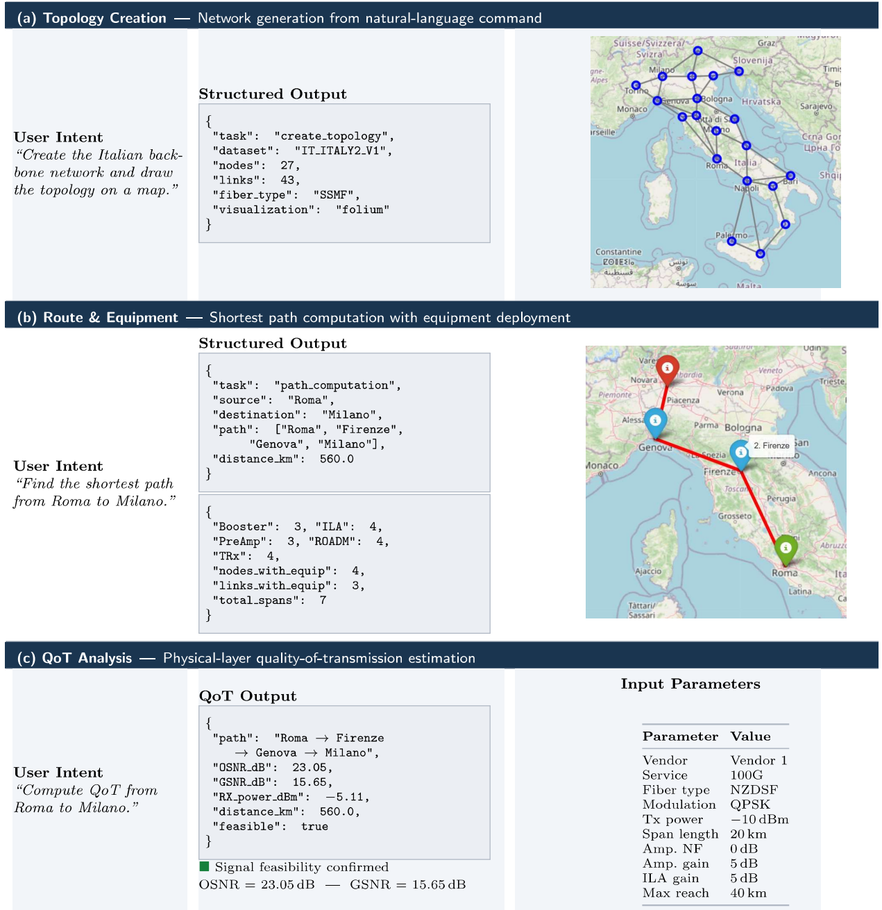
Fig. 2: Demonstration of the LLM-orchestrated Digital twin framework. (a) Topology creation from natural-language input, (b) route provisioning with equipment deployment, and (c) QoT analysis. Structured outputs are shown in the center, with corresponding network visualizations on the right.
