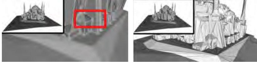
Figure 4.2: Left: a complex 3D model with some distorted elements (e.g., needles) highlighted in the red box. Right: after remeshing, the model can be printed. The original pictures are available in [10].
