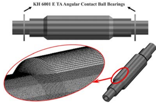
FIGURE 12. 3-D models used for rotor mechanical assessment: Assembled rotor-shaft geometry (top) and finite-element mesh for static-structural analysis (bottom).
