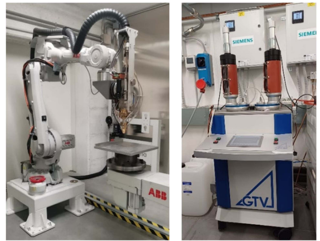
FIGURE 7. DED system used for bimetallic preform fabrication: robotic deposition platform (left) and dual-material powder-feeding system (right).
