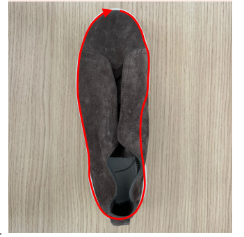
(b) Sequence of the shoe: the unique cutting segment in red.
