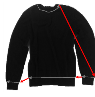
(a) Sequence of the jumper: cutting segments in gray and transition segments in red.
