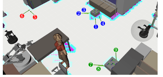
Fig. 6: Sequence of base poses computed to inspect all tags in the environment.
