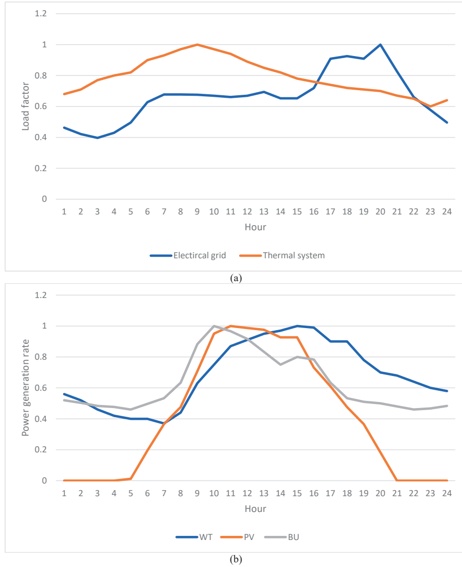
Fig. 4. Expected daily curve for, a) load factor in the different networks [15,27], b) power generation rate of renewable units [27,28].
