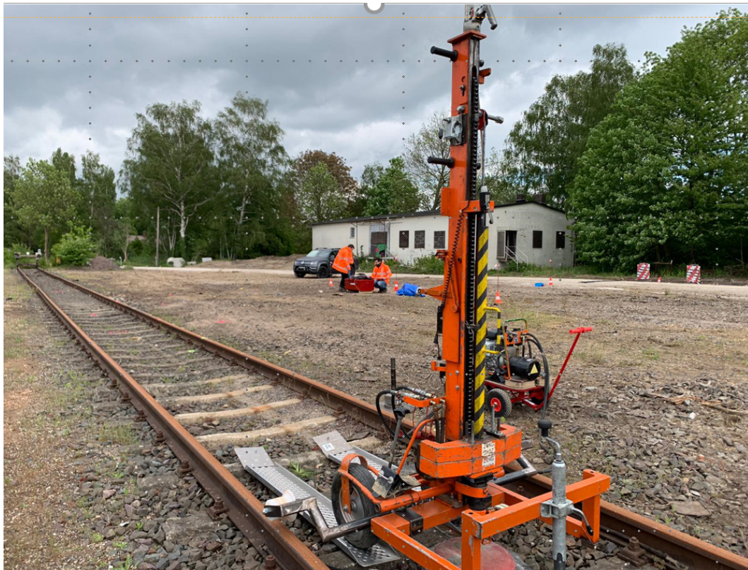
Fig. 2.12 DYNPACT® excitation device used during the in-field measurements. The system consists of a 50 kg drop weight released from a height of 1 m to generate an impulsive load in the soil for mobility and insertion loss evaluation.
