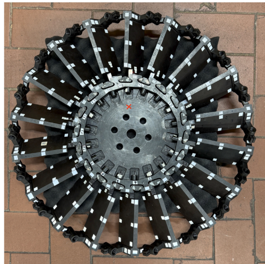
Fig. 9. Full bladed disk assembly. Red cross indicated the excitation point.
