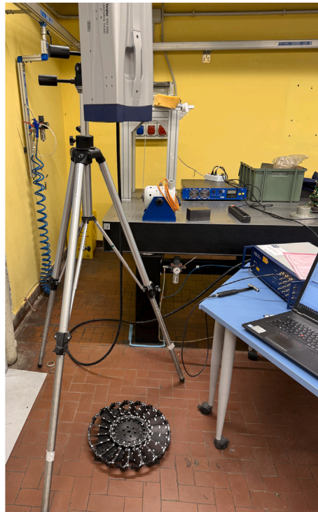
Fig. 2. Experimental setup for modal testing using LDV and impact hammer under free-free conditions.
