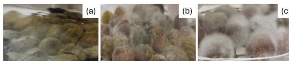
Figure 2. Biomass growth in microcosm at 23 days of incubation: (a) D-W, (b) H, and (c) H-S hazelnuts.
