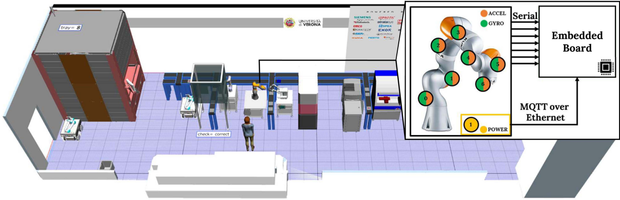
Figure 4. The 3D model of the fully-fledged production line of the ICE laboratory. In the top right corner, we represent the KUKA LBR iiwa and the experimental setup used as case studies.
