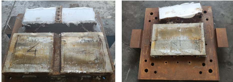
Figure 20 Presence of lubricant on the steel plate as a result of PTFE sliding – unidirectional (left) and multidirectional (right) bearing
