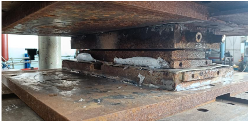
Figure 19 PTFE outflow in the unidirectional bearing after the test
