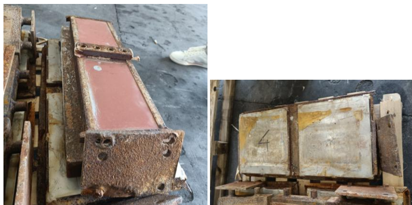
Figure 7 Unidirectional Teflon bearing - upper (left) and lower (right) plates
