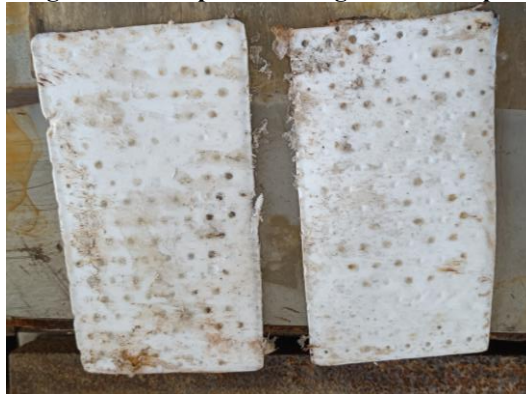
Figure 10 Degradation of Teflon pads
