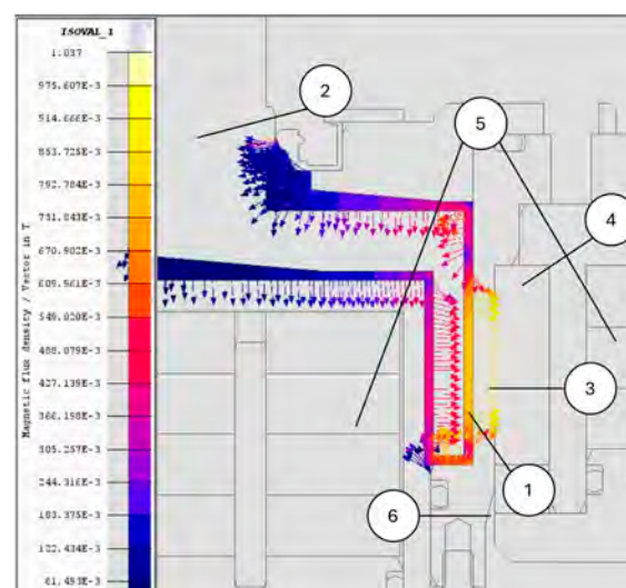
Figure 3. Electro-magnetic simulation—scaled MRB, where: 1—Electric Motor Rotor. 2—Electric Motor Stator. 3—MR Brake Stator. 4—EM Rotor Protuberance. 5—Coils. Arrows represent the direction of magnetic field.
