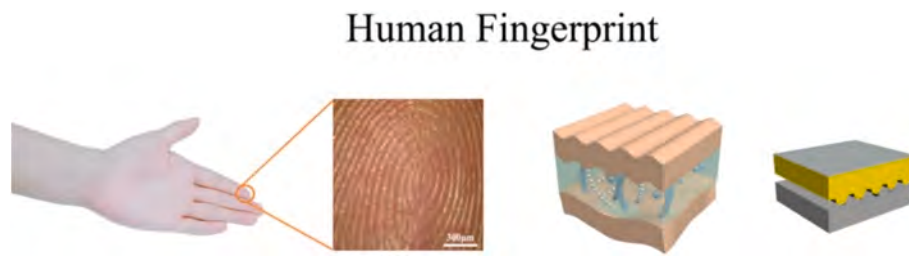
Fig. 27. Example of electronic application of mechanical interlocking structures. Flexible piezoresistive sensor inspired by the structure of human fingerprints, incorporating micro-features between soft-rigid polymers to enhance sensing performance and mechanical stability. Adapted with permission from [137]. Copyright 2024 American Chemical Society.
