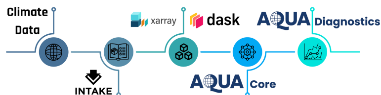
Figure 1. A scheme of the AQUA core dependencies and the separation between the AQUA core and the diagnostics. Climate data are the input for the AQUA code. Intake is then used to create data catalogs. AQUA leverages Xarray and Dask to enable lazy access computation. The AQUA framework is the part devoted to data access and process. Finally AQUA Diagnostics, a diagnostic suite based on the AQUA framework will be introduced in a companion paper.
