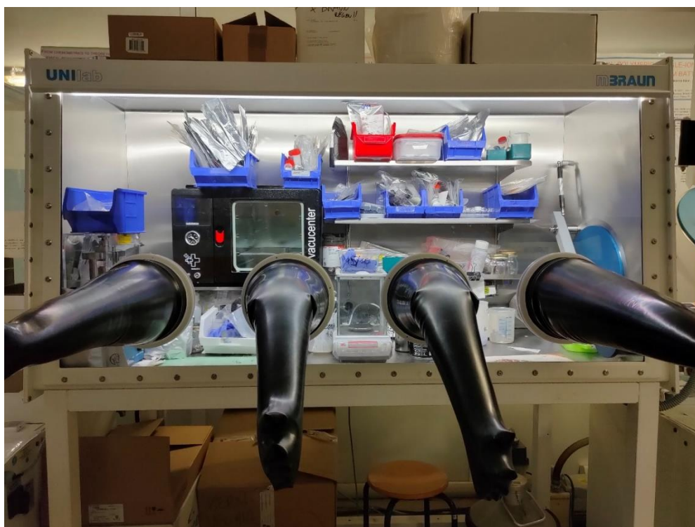
Figure 3.6 Argon-filled glovebox (M-Braun UniLab) used to stock electrolyte and for cell preparation.
