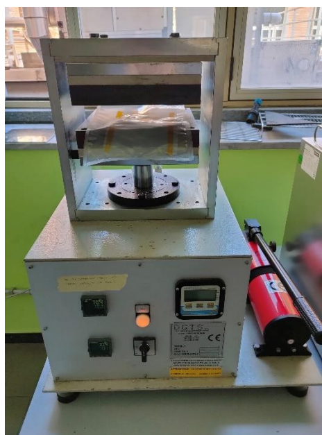
Figure 3.2 Hydraulic press used to heat and press the polymer membrane.
