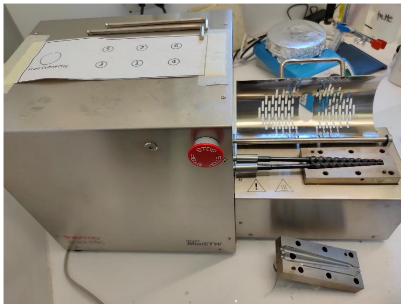
Figure 3.1 Extruder employed for polymer electrolyte preparation.
