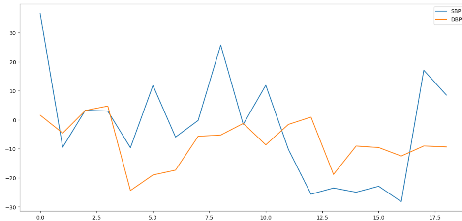
Fig. 5.28 Discrepancies between mean (unweighted) model estimates and external sphygmomanometer values over the 19 PulsECG recordings: \Delta\text{SBP} = -2.33 \pm 17.85 mmHg and \Delta\text{DBP} = -7.67 \pm 7.91 mmHg.
