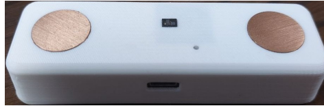
Fig. 5.13 Final PulsECG prototype enclosed in a 3D-printed case.
