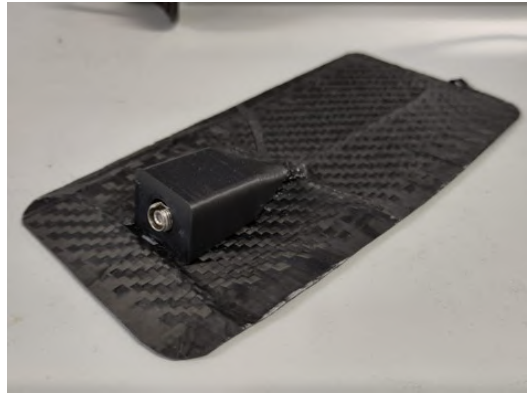
Fig. 8.8 Integrated connector housing and protective structure after assembly.
