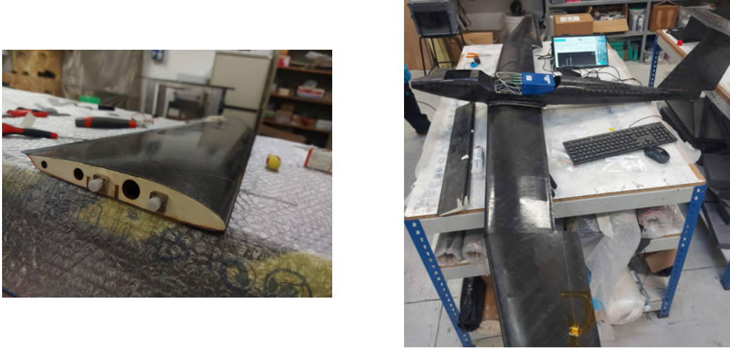
Fig. 13.6 Wing–fuselage interface and first system integration with interrogator.
