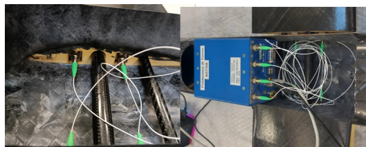
Fig. 13.8 Connection between interrogator and wing-integrated fibers.
