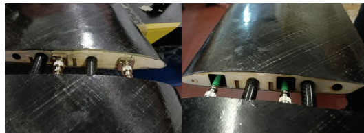
Fig. 13.9 Detail of semi-wing assembly and fiber routing at the interface.
