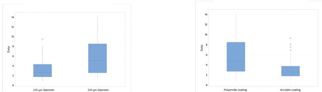
Fig. 7.15 Effect of diameter and coating in nonlinear regime.
