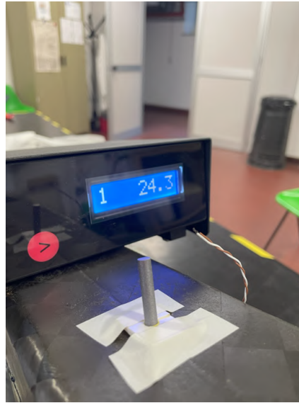
Fig. 12.13 External temperature sensor installation.
