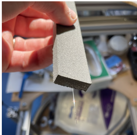
Fig. 8.15 Regolith-based specimen with embedded optical fiber.
