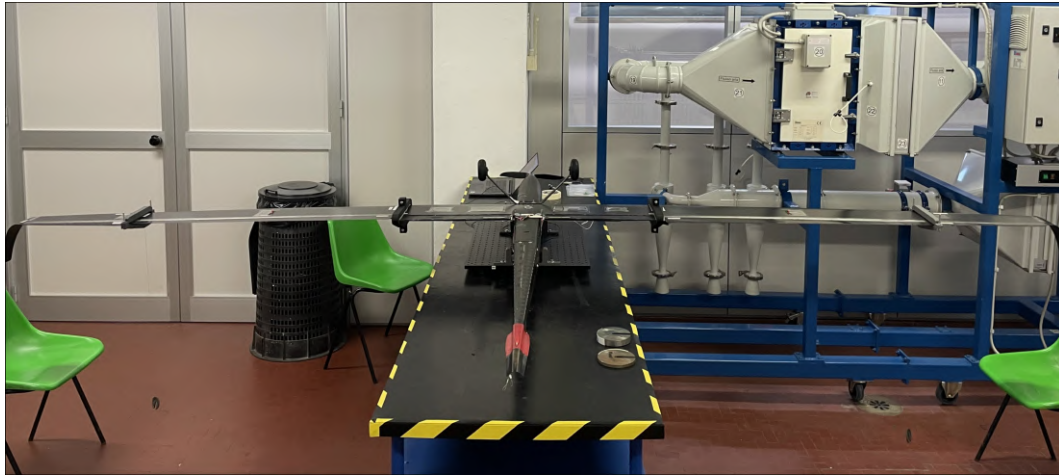
Fig. 12.7 Experimental setup for load-strain calibration.
