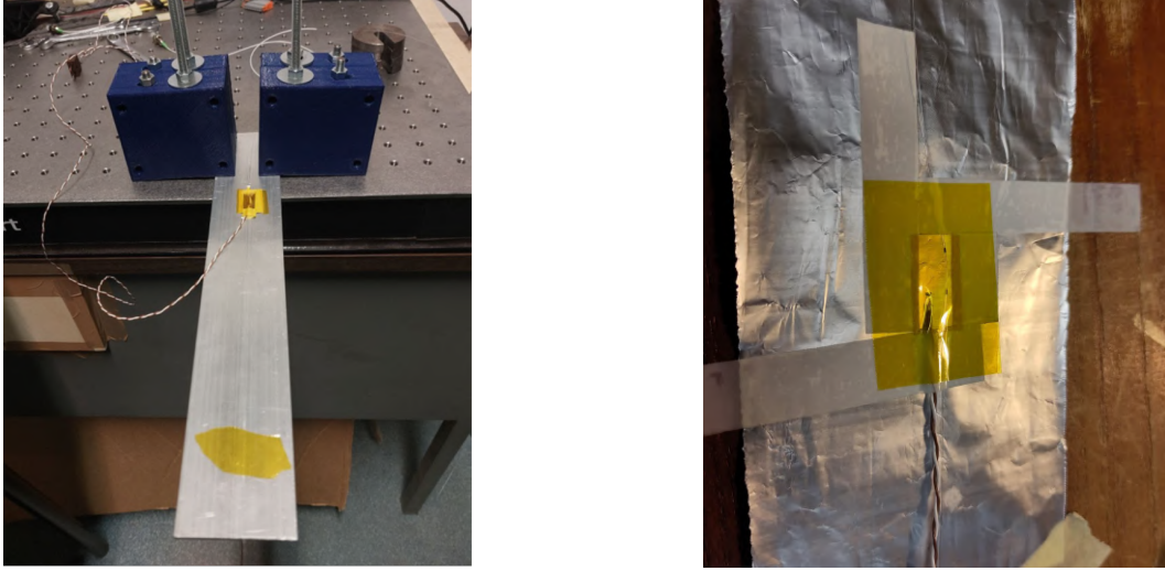
Fig. 4.5 Experimental calibration with FBG and thermocouple.
