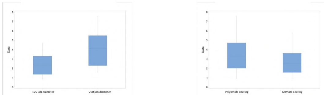
Fig. 7.12 Effect of diameter and coating in linear regime.
