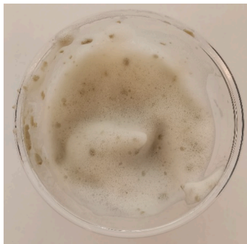
Fig. 6. Foam with clay lumps.
