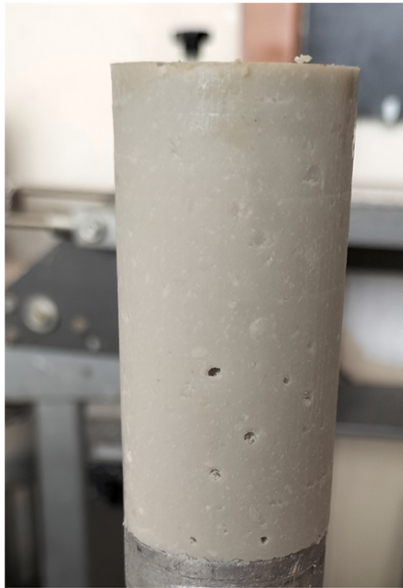
Fig. 3. Photograph showing a triaxial specimen of two-component grout.
