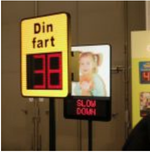
Figure 5: Example of signs relying on infrared or laser sensors for speed control/deterrence
