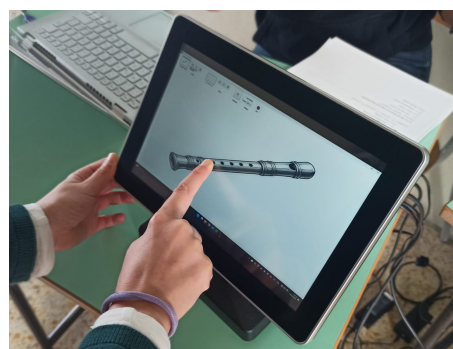
Figure 2: The TanvasTouch haptic interface.
