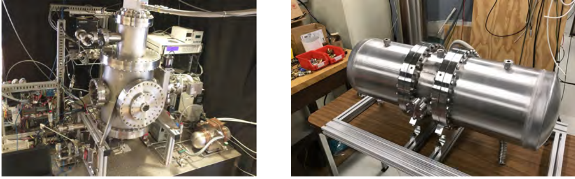
Figure 20. (Left): Test bench for radon adsorption measurement at Columbia University. (Right): In-house developed candidate recirculation pump at the University of California, Los Angeles.
