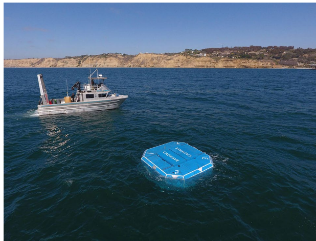
Fig. 7. CalWave's x1™ prototype wave energy converter deployed in 20 m water depth near the Scripps Institution of Oceanography pier in La Jolla, California U.S. (photo credit: CalWave).
