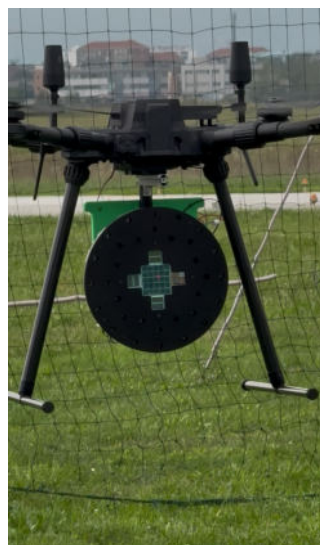
Figure 11. Outdoor validation setup during UAV-assisted calibration of the reference frame transformation.
