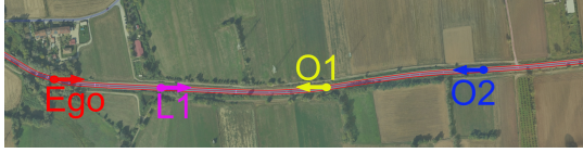
Fig. 4. Overview of the scenario in Roadrunner, detailing the position of the ego vehicle and the actors (L1,O1,O2) before the overtake maneuver.
