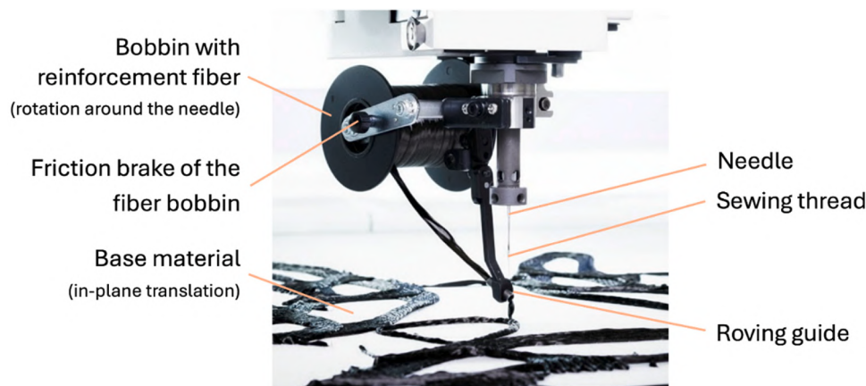
Fig. 1. Stitching process of a TFP preform, showing a carbon fiber roving being stitched over a base material (glass woven).
