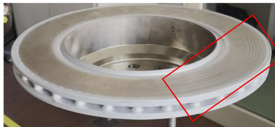
Figure 3. Surface B with damage (i.e. scratch). The red box highlights a part of a physical scratch over the surface.
