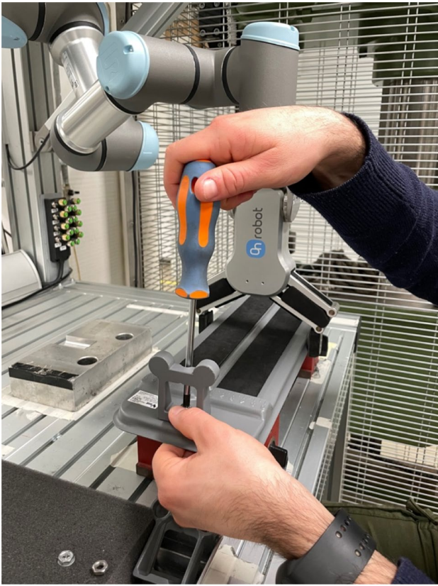
Fig. 2 The UR3e cobot during the collaborative assembly of the tile cutter
