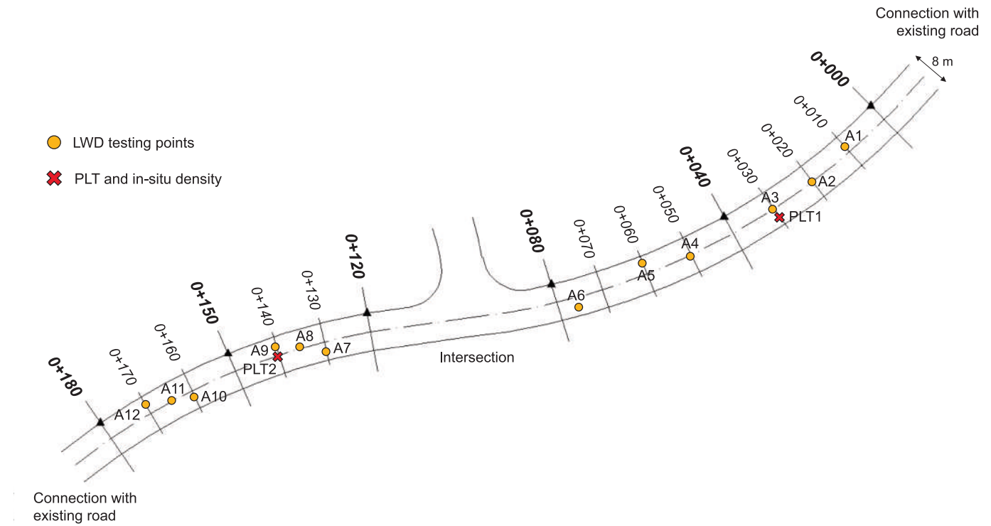
Fig. 9. Location of testing points on the subgrade.
