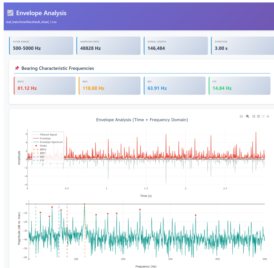
Figure 4. Example of an envelope analysis report: the peaks are consistent with the BPFI and related harmonics, highlighted by markers in the spectrum.
