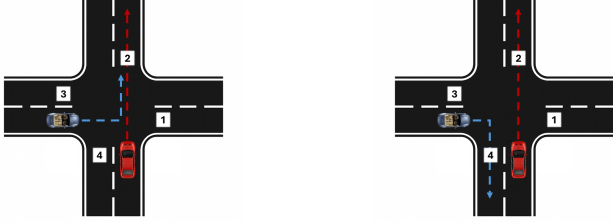
Fig. 4: Potentially interfering actor selection using the intended exit branch index: actors (blue) with b_j^{\text{out}} \leq b_{\text{ego}}^{\text{out}} may cross/overlap the ego vehicle path (red) and are selected; higher-index exits are ignored for this criterion.
