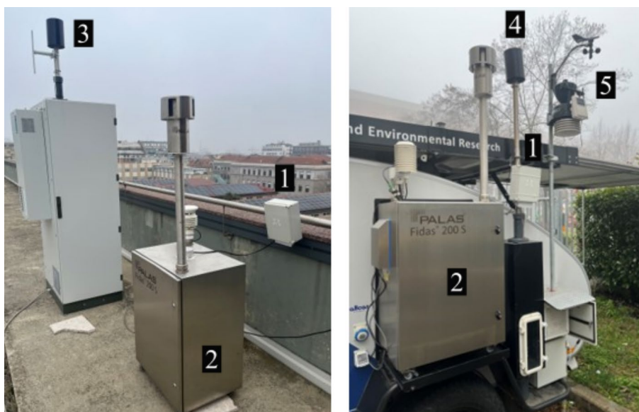
Fig. 2 Positioning of ENEA MONICA microsensors and reference instruments for calibration at DIATI—Politecnico di Torino. Left: CC-Green Roof. Right: CC-TrAIRer Lab. 1—ENEA MONICA™ microsensors, 2—Palas Fidas 200 S optical sensor for PM measurement, 3—Sampling head for ENVEA AC32e analyzer for NO 2 measurements, 4—Sampling head for Serinus 40 analyzer for NO 2 measurements, 5—Davis Vantage Pro 2 weather station
